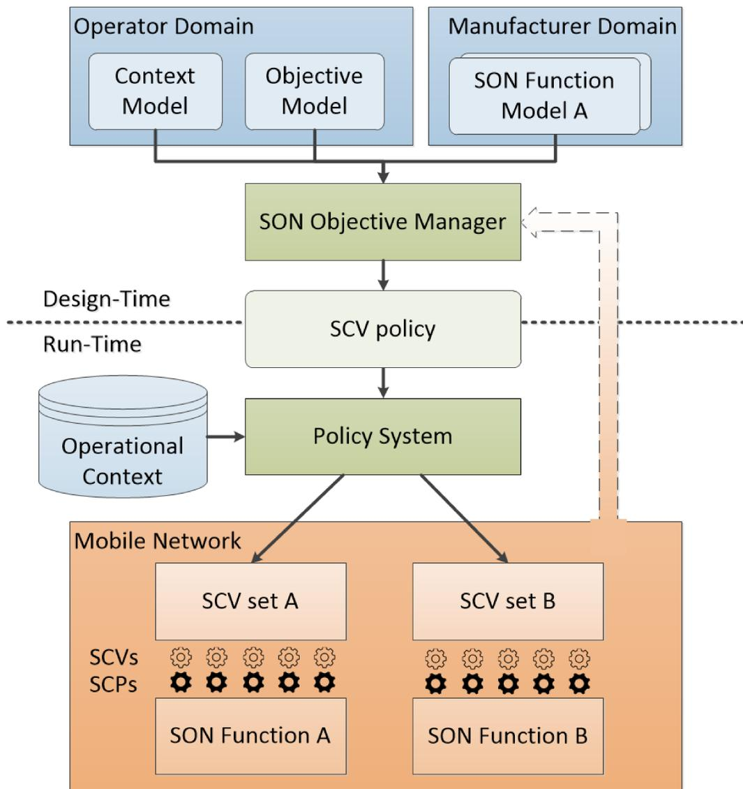
The configuration of the SON with a collection of SCV sets according to a set of technical objectives induces to two *manual gaps*. The human operator has to a) manually translate the objectives into SCV sets, i.e. selecting SCV sets for SON Functions that are in line with the KPI targets, and b) dynamically change the SCV sets according to the operational context, e.g. going from a normal traffic situation into the busy-hour and thus changing operator objectives.
