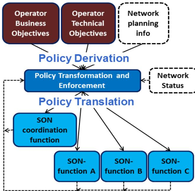
Figure 2: Functional architecture of Policy Transformation and Enforcement.
