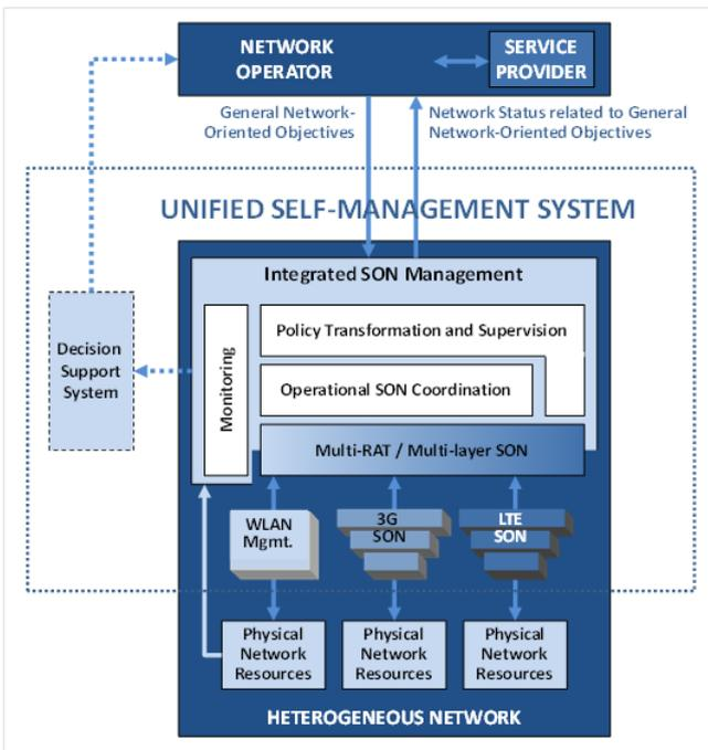
Figure 1: Overview of SEMAFOUR's envisioned unified self-management system.
