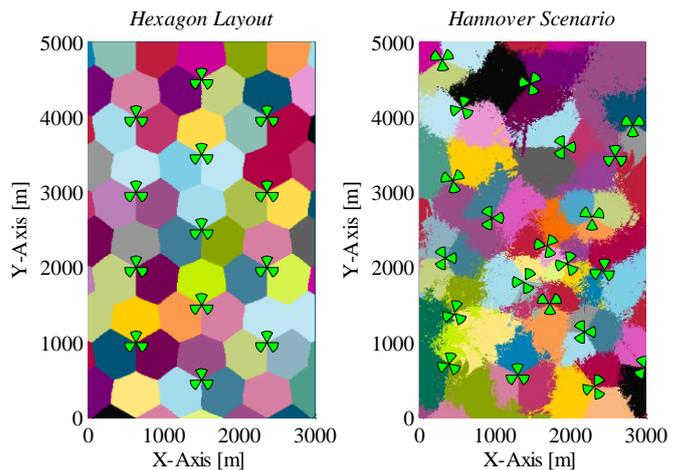
Figure 3: Best-Server-Map of the Simplified Hexagonal Network (left) and the Realistic Urban Hannover Scenario (right)
