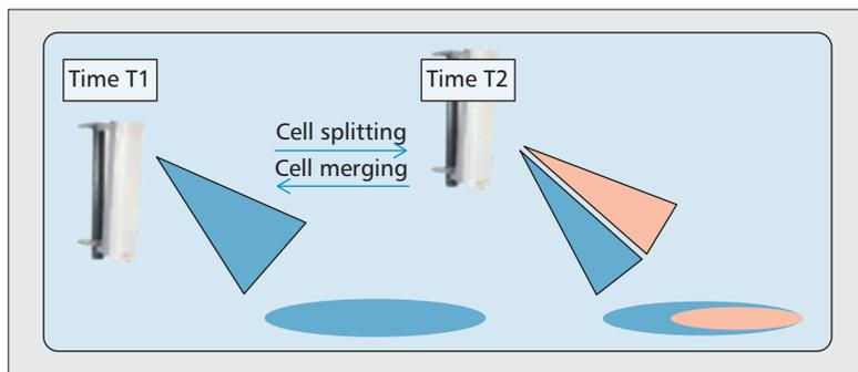
Figure 4. Changing cell pattern of active antenna.
